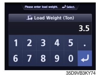
Enter load weight using up or down buttons.
