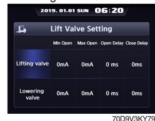
For each valve value, you can adjust the current value and time on the above screen
