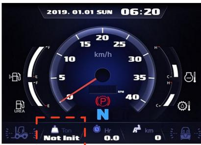
· Truck that has applied the weight sensor (option)
